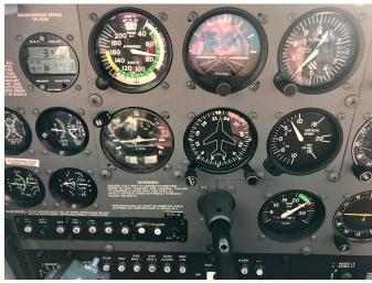
Spot the difference. Both of these pics were taken in 2SP. The left photo was taken on 12/26; the right one on 7/7. Both were taken on departure RWY 22 at N51, at 300'-400' AGL and within a couple knots. Look at the climb rate then check the OAT for the explanation.
