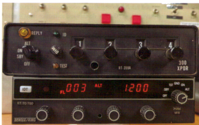
An ATC radar beacon transponder sits on top of a Mode S transponder.
