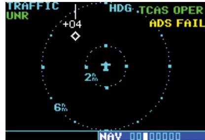
**Traffic With GDL 88/ADS-B With TCAS Operating and ADS-B Failed**
