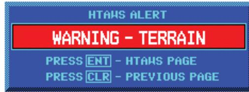
**FLTA WARNING**— Warning pop-up alerts are issued 15 seconds prior to an estimated potential impact in normal mode and approximately 10 seconds in RP Mode. FLTA warning alerts are accompanied by the aural message “*Warning - Terrain, Terrain*”. Similarly, a “*Warning - Obstacle, Obstacle*” alert is also provided. The time to an alert can vary with conditions, therefore there is no guarantee of a 15/10 second warning alert being issued.
