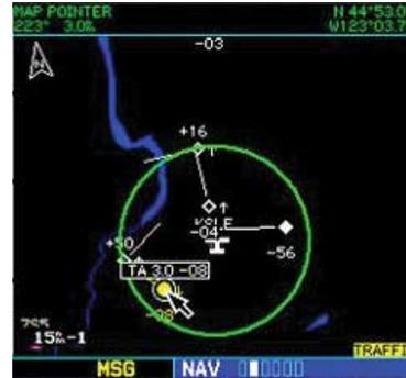
When the target pointer is placed on traffic, the traffic range and altitude separation are displayed.
