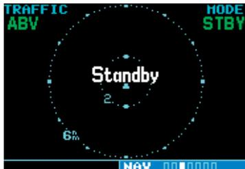
The Standby Screen appears when the GTS 8XX series passes the power-up test.
