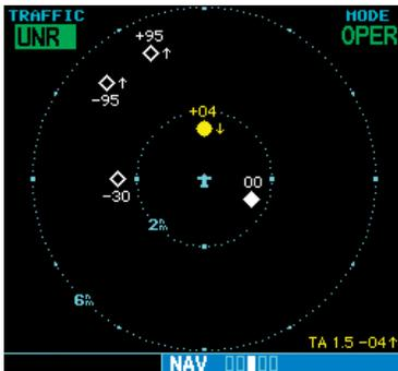
The name of the selected altitude display mode (ABV: look up, NRM: normal, BLW: look down, or UNR: unrestricted) is displayed in the upper left-hand corner of the Traffic Screen. The GTS 8XX series continues to track up to 30 intruder aircraft within its maximum surveillance range, regardless of the altitude display mode selected.
