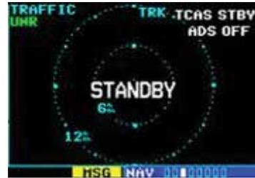
The Standby Screen appears when the ADS-B passes the power-up test.
