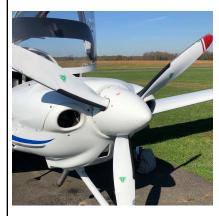
\*Both aircraft should be left with one blade pointed down at 6-o'clock. (This allows precipitation to drain out of the spinner. preventing ice damage.)
