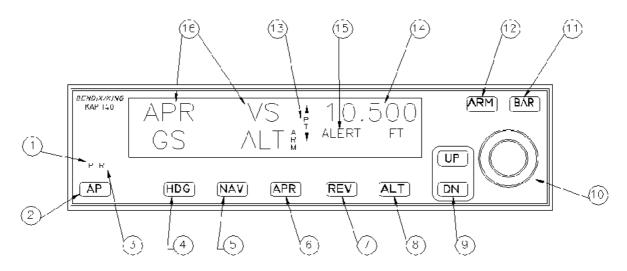
1. PITCH AXIS, (P) ANNUNCIATOR - When illuminated, it indicates failure of the pitch axis and will either disengage the autopilot or does not allow engagement of the pitch axis. The P light may illuminate with the autopilot disengaged. This condition can occur during maneuvering flight when g thresholds are exceeded. The autopilot monitor will not allow engagement during illumination.
